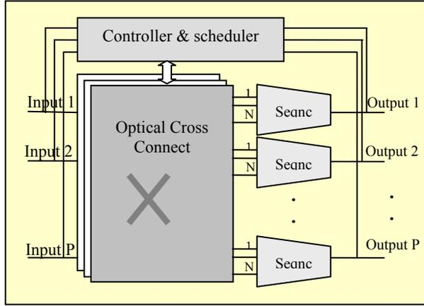
Figure 1 – Switch Architecture
