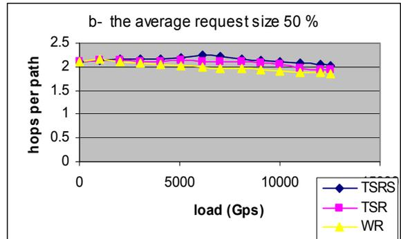
Figure 8 - average number of hop versus the load for TSRS, TSR and WR
